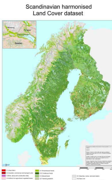
Figure 1: Harmonised Scandinavian Land Cover dataset from aggregated national data from Norway, Sweden and Finland (1 ha minimum mapping unit; 21 thematic classes). © ETCLUSI - UAB
